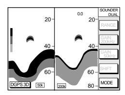
Figure 2-13 Dual-frequency display
